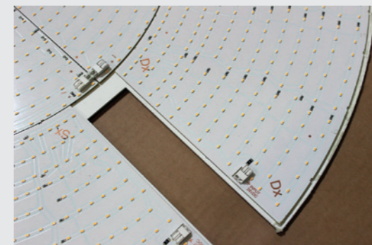
Piastra LED custom / Custom LED board: 160 W , 18400 lm 2700 K , CRI: 90
