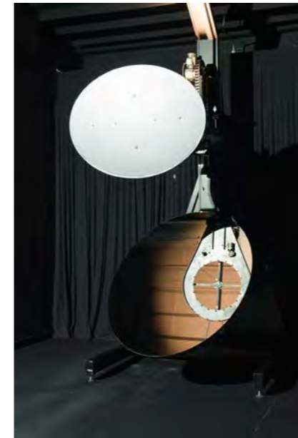
Photometric Measurements - Goniophotometer with rotating mirror
