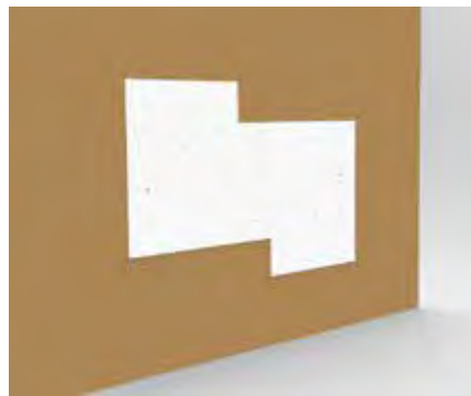
2. Use the provided template to drill the holes and paint the drywall.
