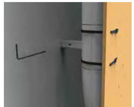
6. Detail of the wall pins fixing.
